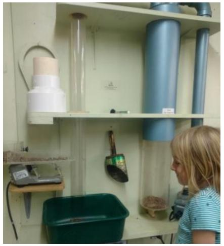
Figure 41. Air separator to remove debris and unfilled seeds.
